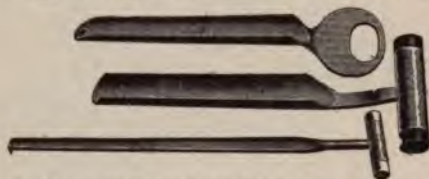
Fig. 220. Two cheese-tries and one butter-tryer (the longest one).
